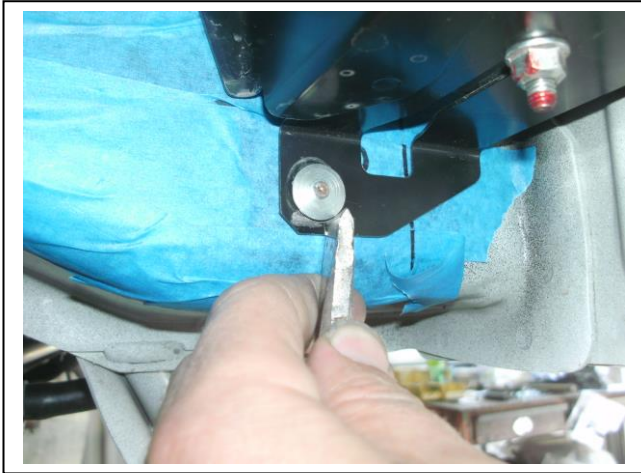
Figure 1: Using chisel to place cut in edge of security bolt.
