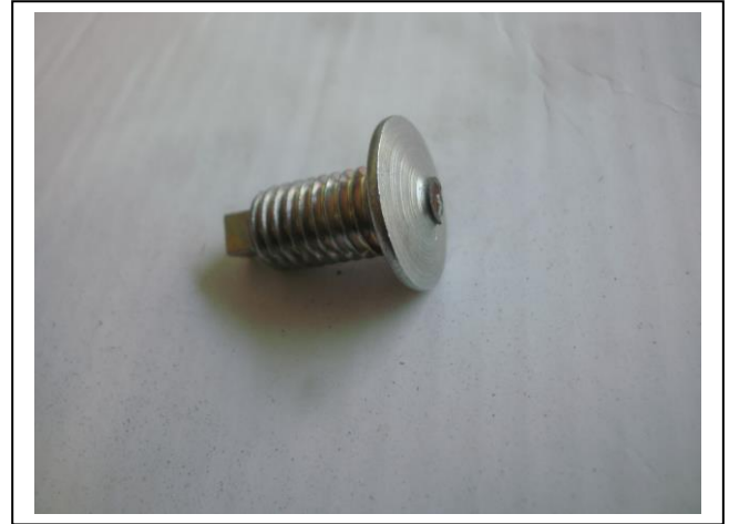
Figure 2: View of security bolt when removed from vehicle.
