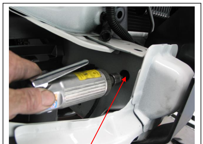
Figure 6 Enlarging outer chassis hole to 17mm for chassis spacer
