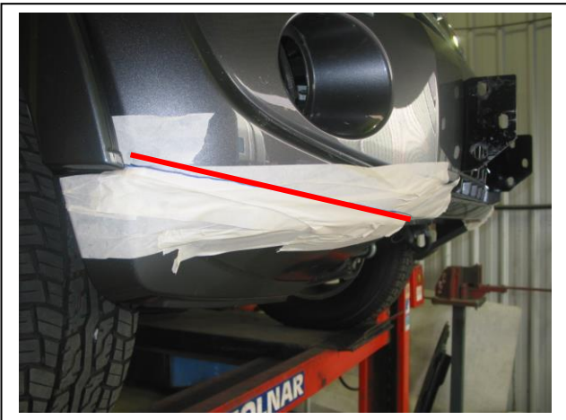
Figure 9: Cut line from flare to inner corner of plastic bumper cover.
