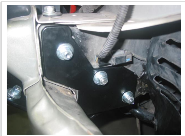
Figure 5: Placement of outer chassis washer
